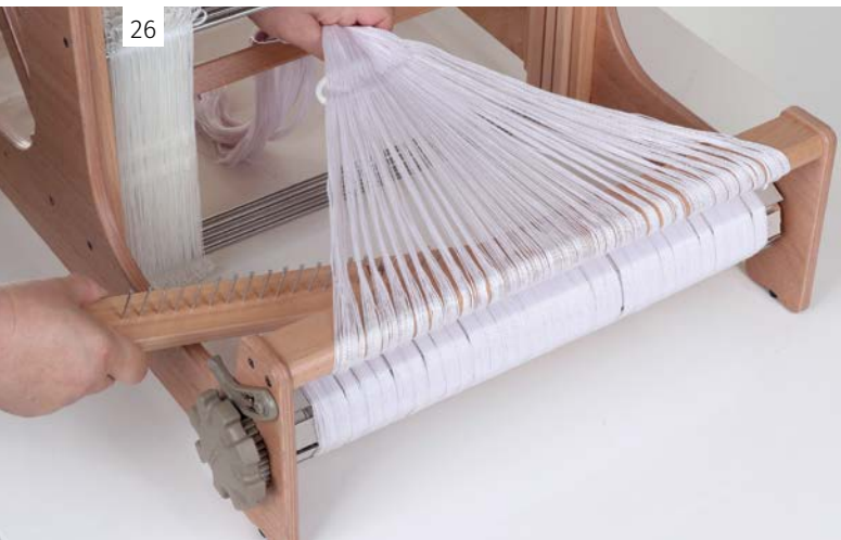
26 Drop the raddle down from the warp.
